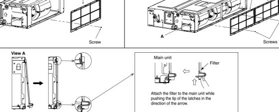
Attach the filters (accessories) in the manner shown in the figure. Securely fix the filters with the screws.
