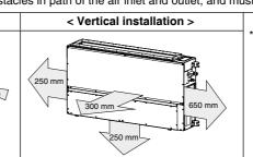
t is necessary to make space for the cleaning as well as the maintenance of the drain pan and the heat exchanger. Do not put any obstacle not to cause obstructing maintenance or cleaning works If the place where the ceiling material cannot be removed, make an opening section below the bottom surface of the indoor unit in order to take it out If it is impossible to provide an opening, make space more than 300 mm between the indoor unit's bottom surface and the ceiling material.
