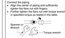
Seal sufficiently the flare nut (both gas and liquid sides) with neutral cure (Alkoxy type) & ammonia-free silicone sealant and insulation material to avoid the gas leak caused by freezing. \* Use of silicon containing ammonia can lead to stress Apply neutral cure (Alkoxy corrosion on the joint & can cause leakage. type) and ammonia-fre silicone sealant along the Neutral cure (Alkoxy type) & ammonia-free silicone
